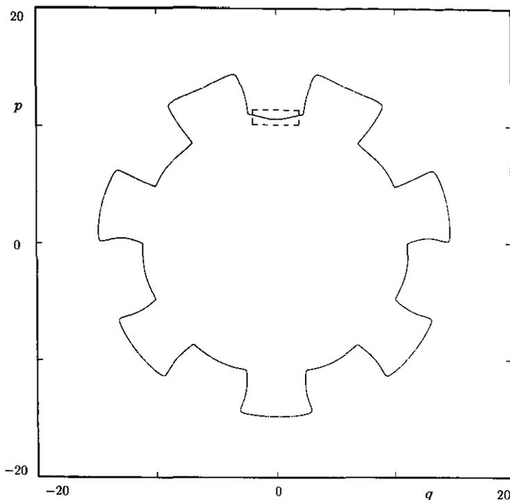
**Figure 5.**  $H = \frac{1}{2}(p^2 + q^2) - \epsilon \cos(q - 7t)$ . Part of an orbit on the chaotic web formed by separatrix splitting (see figure 7). The initial condition is  $(q_0, p_0) = (0, 10.5939)$  and there are  $m = 4$  time steps per forcing period. The Poincaré map is shown for 25 000 periods. The orbit stays on the same two separatrix levels.
