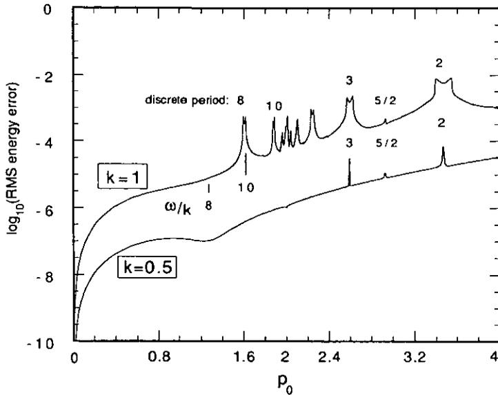
Figure 4. Effect of time step resonances. Here we integrate the pendulum with the optimal fourth-order method for initial conditions  $(0, p)$ ,  $0 < p < 4$ . The RMS energy error up to  $t = 2000$  is shown.
