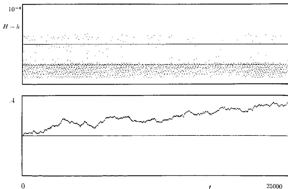
**Figure 8.** Energy error for coupled pendula.  $H - h$  is the change in energy from that at the initial condition,  $k = 0.5$ : (a) initial condition  $(0, 2)$  (near elliptic periodic orbit); (b) initial condition  $(2, 2)$  (chaotic orbit). Note the different vertical scales.
