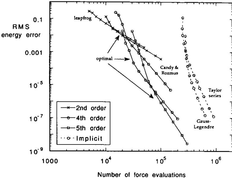
**Figure 3.** Relative efficiency of different methods. See caption for figure 2. Each implicit method requires two trigonometric function evaluations per iteration in this case; we have counted this as two force evaluations.
