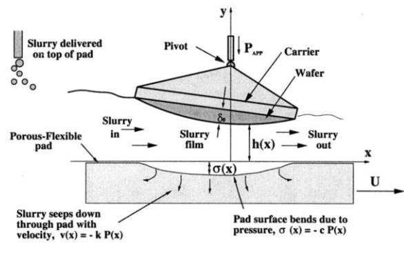
Fig. 2. Model schematic for slurry delivery on top of pad.
