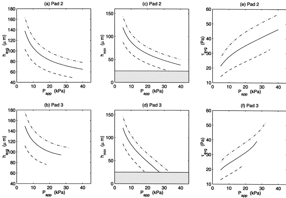
Fig. 5. Effect of  $P_{app}$  and  $U$  ( $U = 0.5$  m/s, (---);  $U = 1.0$  m/s, (—);  $U = 1.5$  m/s, (-·-·-)) on  $h_{avg}$ ,  $h_{min}$ , and  $\tau_{avg}$  for pad 2 and pad 3 (slurry delivered on top of pad). Other parameters used for the above computations are:  $D = 8$  in,  $\delta_0 = 10$   $\mu\text{m}$ ,  $\mu = 0.003$  Pa s. Slurry delivery is on the top of pad in all cases shown.
