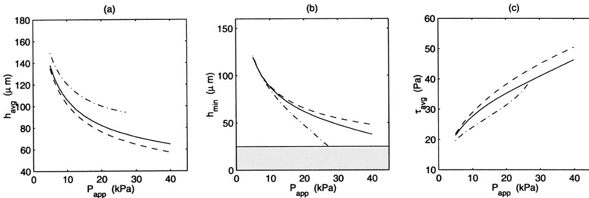
Fig. 6. Comparison of  $h_{avg}$ ,  $h_{min}$ , and  $\tau_{avg}$  (a–c) for pad 1 (---), pad 2 (—), and pad 3 (-·-·-) for different values of  $P_{app}$ . Other parameters used for the above computations are:  $U = 1$  m/s,  $D = 8$  in,  $\delta_0 = 10$   $\mu\text{m}$ ,  $\mu = 0.003$  Pa s. Slurry delivery is on the top of pad in all cases shown.
