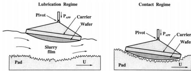
Fig. 1. Lubrication and contact regime of CMP.
