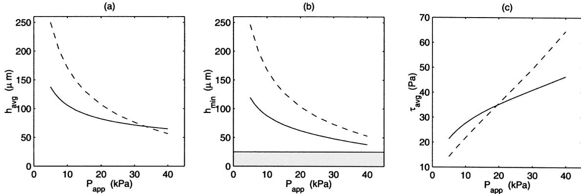
Fig. 7. Comparison of  $h_{avg}$ ,  $h_{min}$ , and  $\tau_{avg}$  (a–c) for slurry delivery from top (—) and bottom (---) using pads 2 and 4, respectively. Other parameters used for the above computations are:  $U = 1$  m/s,  $D = 8$  in,  $\delta_0 = 10$   $\mu\text{m}$ ,  $\mu = 0.003$  Pa s. Note: A pad with holes is used when the slurry is delivered from the bottom. Slurry is delivered at a constant rate of 1 mm/s at all  $P_{app}$  for pad 4.
