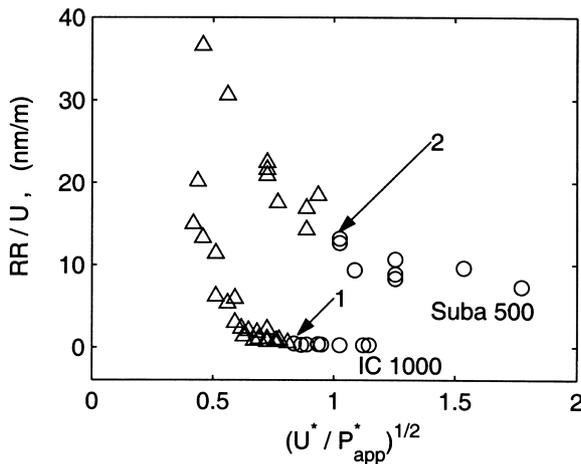
Fig. 8. Plot of normalized removal rate,  $RR/U$ , against  $(U^*/P_{app}^*)^{1/2}$  for IC 1000 and Suba 500 pads, where  $U^* = U/U_{ref}$  and  $P_{app}^* = P_{app}/P_{ref}$ , with  $U_{ref} = 1$  m/s, and  $P_{ref} = 20$  kPa. The triangle and circle symbols show the contact and lubrication regimes, respectively. The arrows mark the transition into the lubrication regime.
