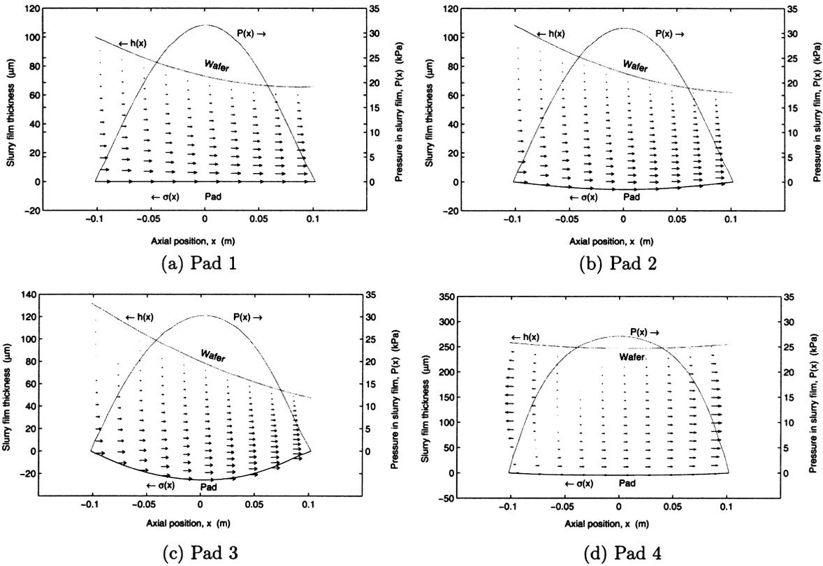
Fig. 4. Slurry velocity and pressure distributions, pad and wafer positions for pads 1–4 at base case parameter values given in Table 1 are used.  $P_s = 30$  kPa for pad 4.
