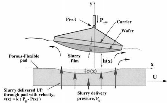
Fig. 3. Model schematic for slurry delivery up through pad.
