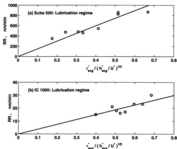
Fig. 9. The removal rate,  $RR$ , is proportional to  $\tau_{\text{avg}}^*/(h_{\text{avg}}^*/U^*)^{1/3}$  for both (a) Suba 500, and (b) IC 1000 pads in the lubrication regime. The (\*) represents dimensionless quantities:  $\tau_{\text{avg}}^* = \tau_{\text{avg}}/\tau_{\text{ref}}$ ,  $h_{\text{avg}}^* = h_{\text{avg}}/h_{\text{ref}}$  and  $U^* = U/U_{\text{ref}}$ , with  $\tau_{\text{ref}} = 40$  Pa,  $h_{\text{ref}} = 25$   $\mu\text{m}$ , and  $U_{\text{ref}} = 1$  m/s.
