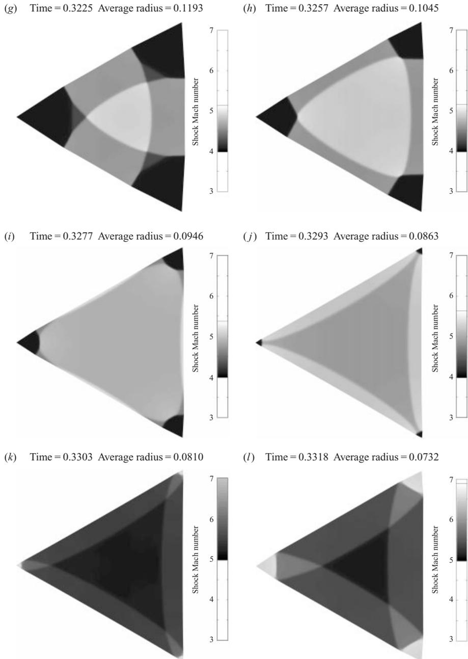
FIGURE 9 (g-l). Shock surfaces in a converging channel with  $\phi = 20^\circ$ : repeating behaviour.
