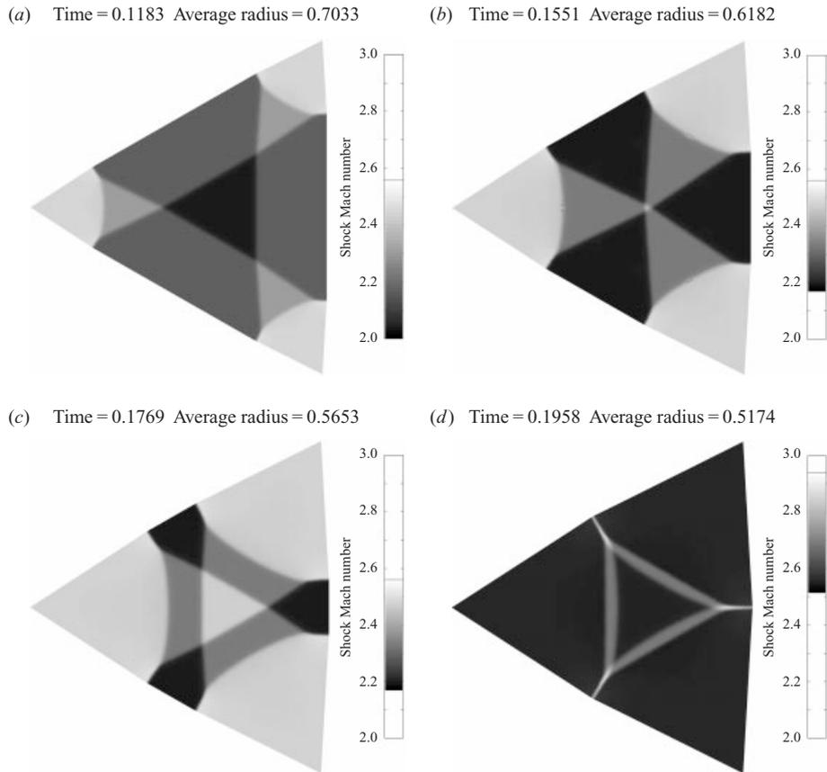
FIGURE 7. Shock surfaces in a converging channel with  $\phi = 20^\circ$ : early behaviour.
