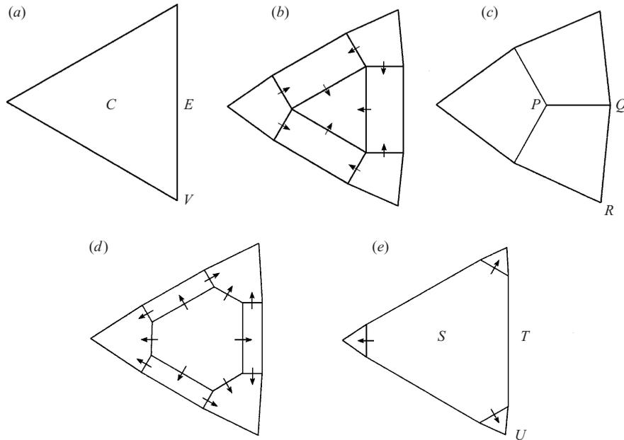
FIGURE 4. Top view of the successive shock surfaces in a converging channel corresponding to the construction in the cut planes shown in figure 3. (The contraction in scale is not shown in the figure.) The arrows indicate the direction of propagation of the shock-shocks.
