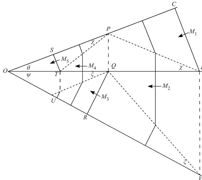
FIGURE 3. Behaviour of a converging shock in the cut planes  $OCE$  and  $OEV$ .
