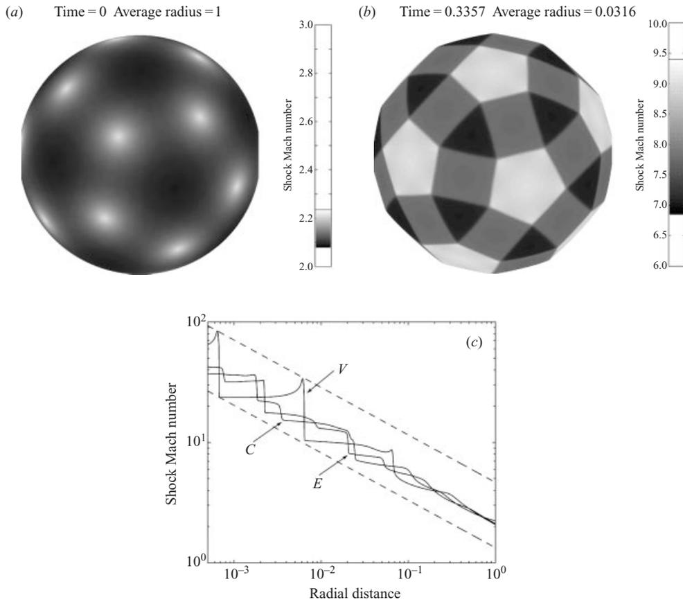
FIGURE 11. Converging spherical shock subject to smooth symmetric perturbation: (a) shock surface at  $t = 0$ , (b) shock surface at  $t = 0.3357$ , and (c) shock Mach numbers along rays.
