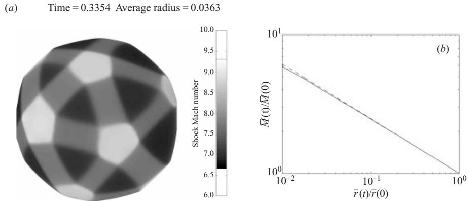
FIGURE 12. Converging spherical shock subject to a smooth asymmetric perturbation: (a) shock surface at  $t = 0.3354$  and (b) average shock Mach number versus average radius.
