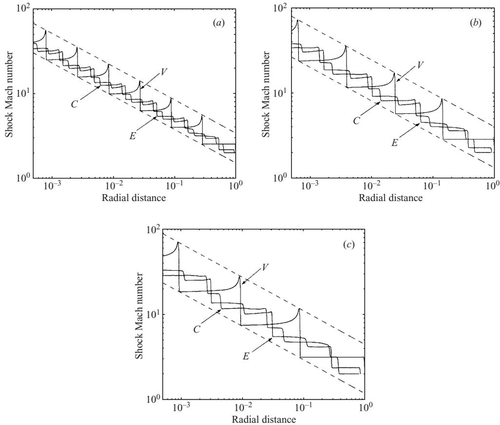
FIGURE 10. Behaviour of the shock Mach numbers along rays from the points  $V$ ,  $E$  and  $C$  for (a)  $\phi = 20^\circ$ , (b)  $\phi = 30^\circ$  and (c)  $\phi = 37.38^\circ$ .
