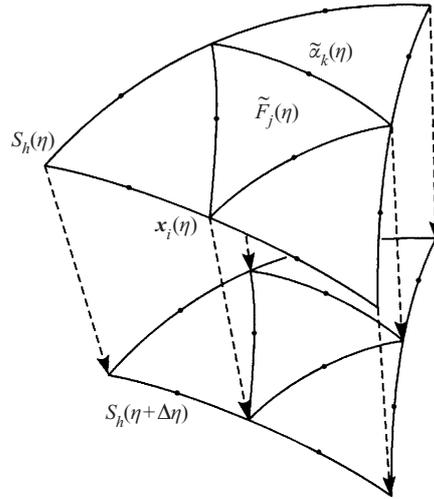
FIGURE 6. A small portion of the unstructured grid on surfaces  $S_h(\eta)$  and  $S_h(\eta + \Delta\eta)$ .
