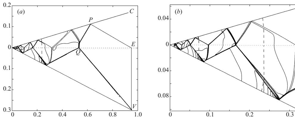
FIGURE 8. Contours of Mach number in the planes  $OCE$  and  $OEV$  for shock propagation in a converging channel with  $\phi = 20^\circ$ .
