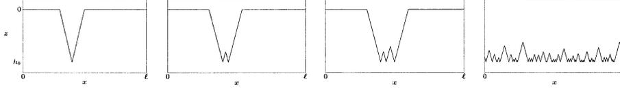
Figure 4. A typical sequence of solid pad-surface profiles after successive steps of the discrete conditioning process (2.4), for  $n = 1, 2, 3$ , and  $n = 50$  with an initially flat pad-surface.
